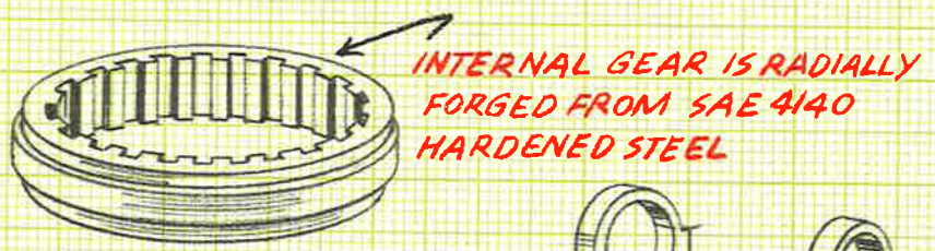
SPLINES ARE RADIALLY FORGED ON CYLINDRICAL END OF FORGED PART
