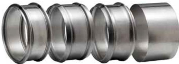
Sizing and forming applications for the automotive industry such as wheel rims, brake drums and emission shells. These emission shells are first profiled on a Grotnes Roll Former. After profiling, the shells are calibrated on a Grotnes Expander.
