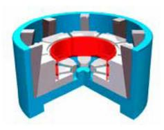
When the part reaches the desired shape and dimensions the pressure ring retracts, the shrinker jaws and dies return to the original position, and the formed part is removed from the machine.
