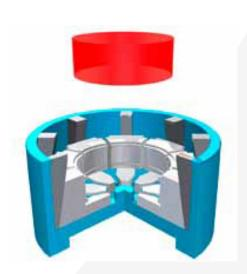
When the dies meet the wall of the part, they exert sufficient force to form the part in a new size and shape as dictated by the dies.
