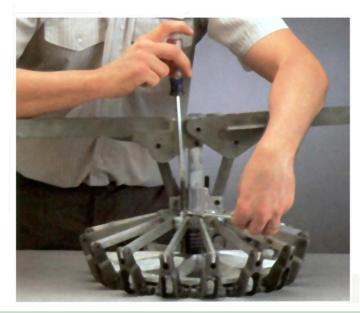
Adjustment is provided by means of two adjusting bolts for varying the amount of closure.
